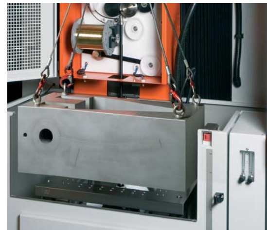
Large UV travel to facilitate loading by hoist
