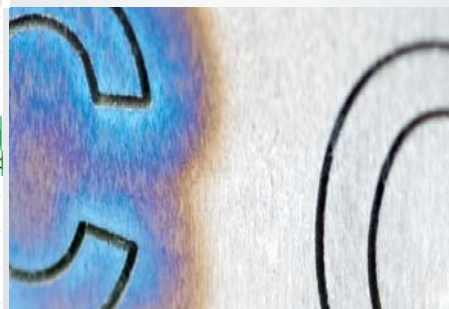
Surface machined with a conventional generator: deposits, pollution
