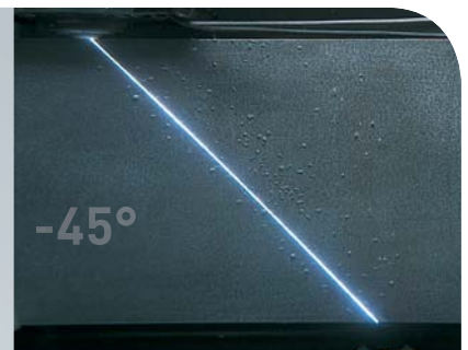
Machining in taper mode of -45° to +45° of the whole height of the part (as an option)
