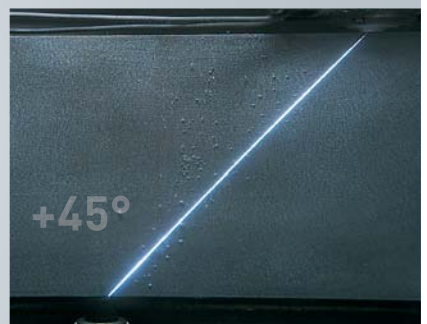
Machining in taper mode of -45° to +45° of the whole height of the part (as an option)
